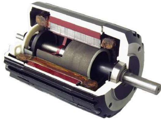
Fig. 3-13A: Cutaway view of Bodine type 34B, brushless DC motor with built-in commutator, and permanent magnet rotor.
